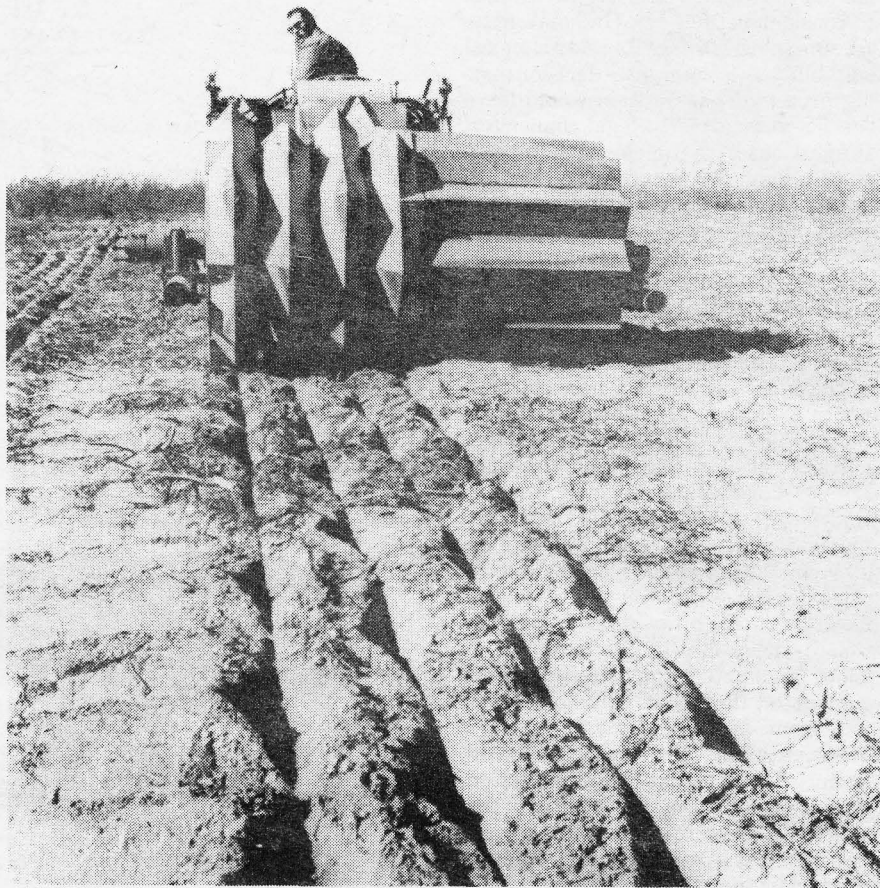
A rolling rangeland imprinter operating on severely overgrazed land near Tombstone, Arizona. The resulting angular depressions in the soil surface funnel rainwater, litter, seeds, and topsoil together where they can work in concert to germinate seeds and establish seedlings. Photo courtesy of Ann Carr.
